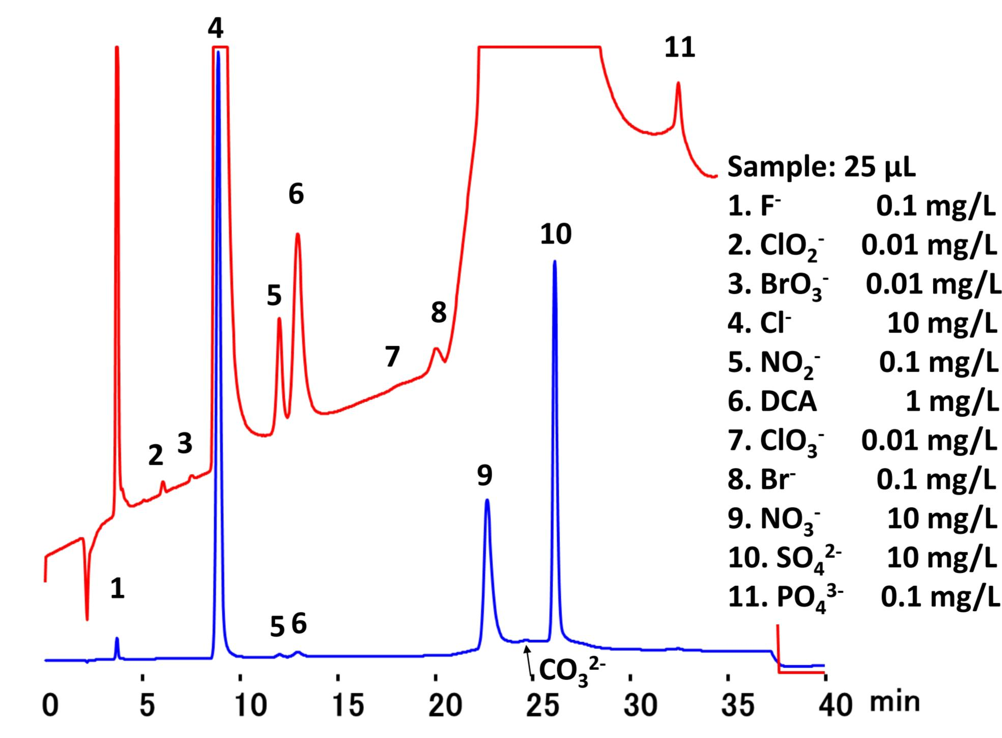
Column: Shodex IC SI-36 4D (4.0 mmI.D. x 150 mm)
