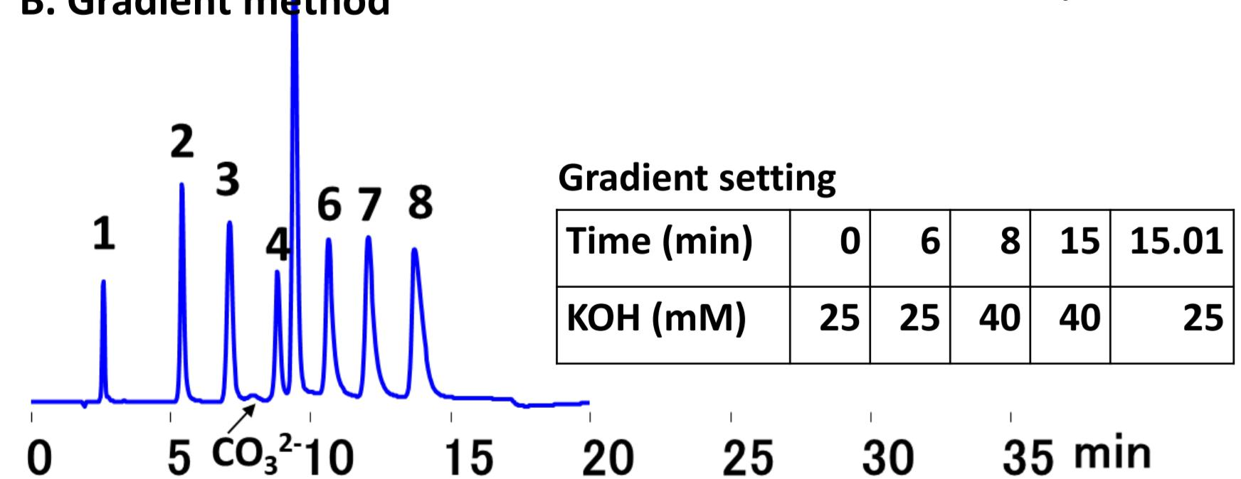
Column: Shodex IC SI-36 4D (4.0 mmI.D. x 150 mm)
