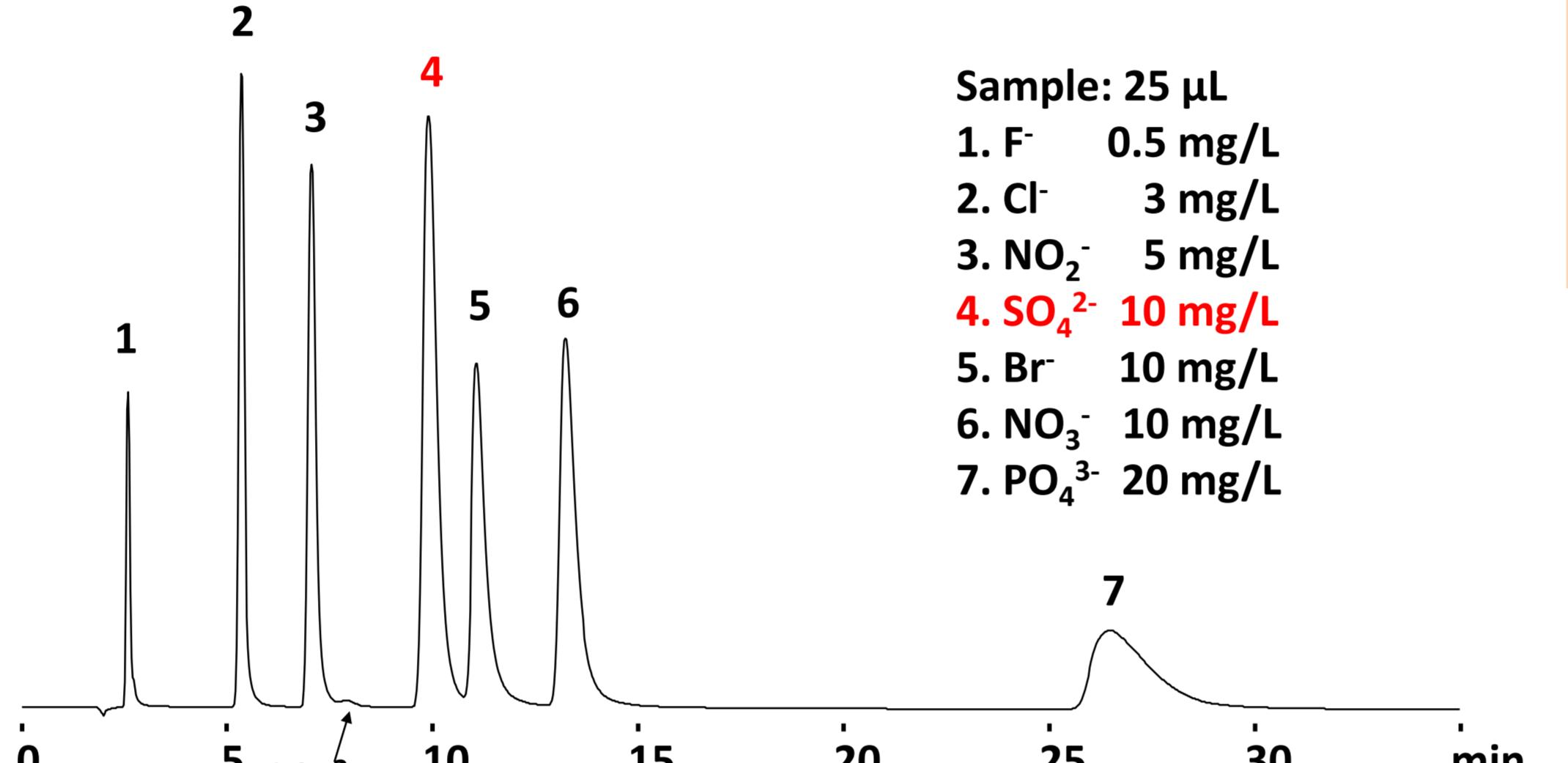
IC SI-36 4D uses potassium hydroxide aqueous solution for the analysis of anions.
