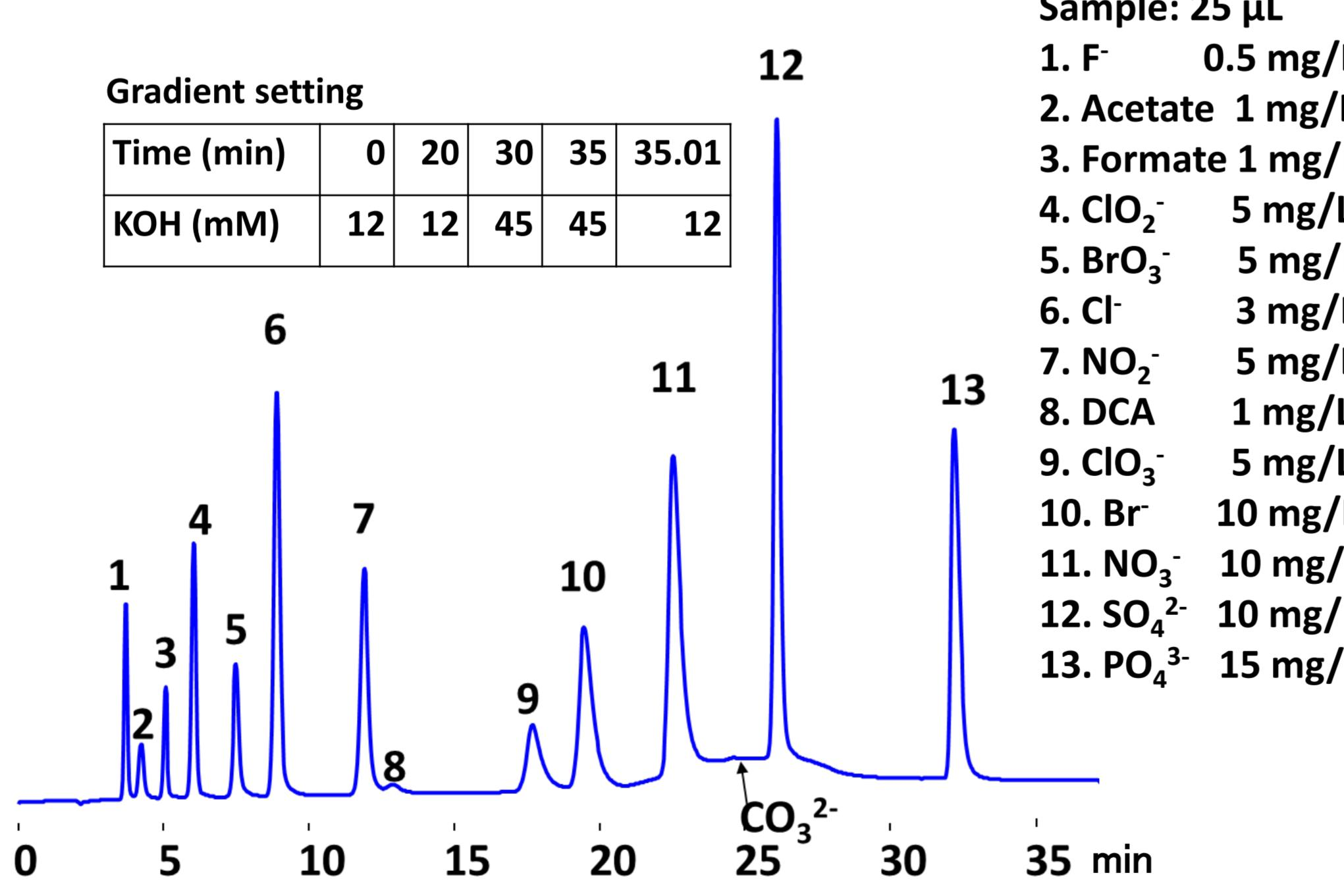
Column: Shodex IC SI-36 4D (4.0 mmI.D. x 150 mm)
